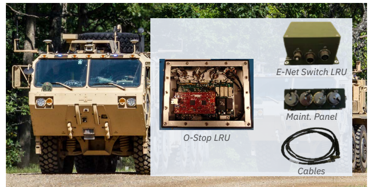
Warfighter machine interface/radio network interface (WMI-RNI) components fabricated for Leader-Follower
